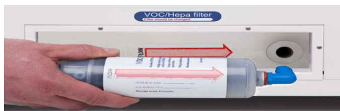
Figure 12.2 The direction of pulling the filter
