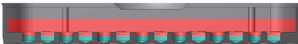
Figure 21.4 The culture wells are covered with a mineral oil layer, and the lid is put on
