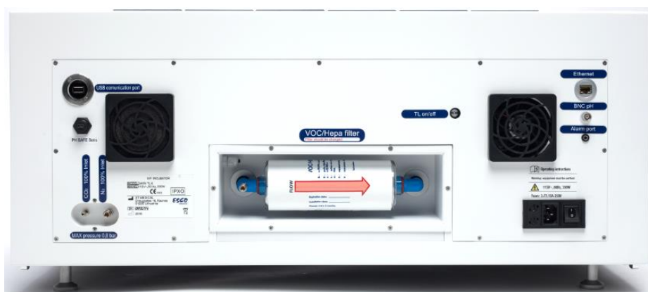
Figure 13.1 MIRI® TL6 multiroom IVF incubators rear
