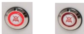
Figure 14.1 Alarm key which indicates the alarm condition
