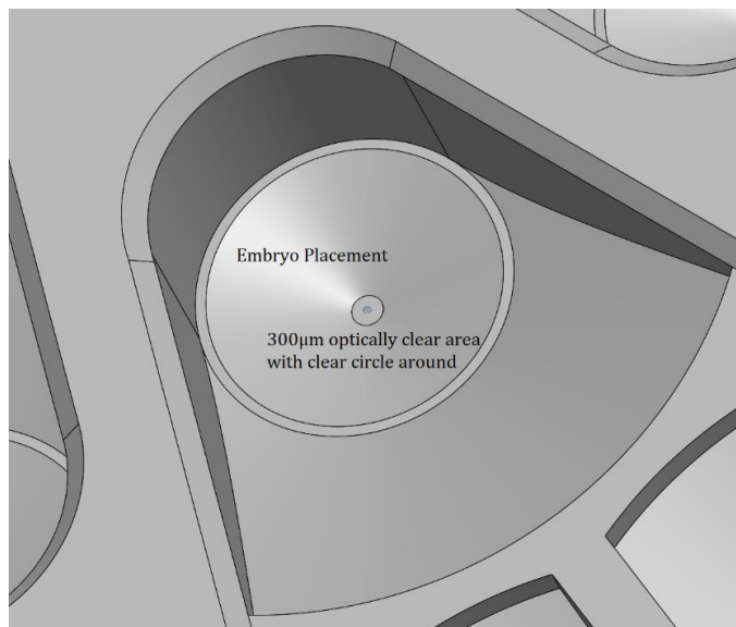
Figure 21.3 Embryo Placement in detail on the 300 \mu\text{m} optically clear area
